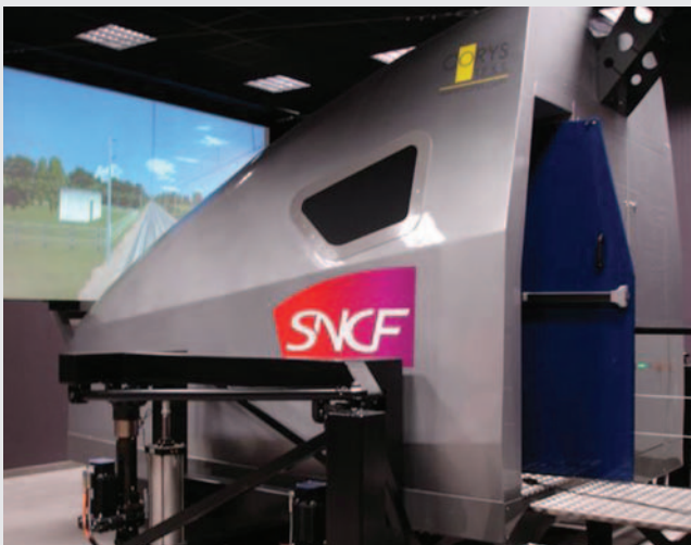
Corys TGV simulator that will be used to train drivers on the new TGV route between Paris and Strasbourg
